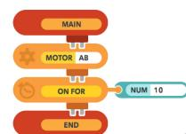
This program tells motors A and B to run for one second.
