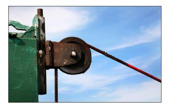
A pulley is a simple machine made with a rope or belt wrapped around a grooved wheel. Pulleys are generally used to raise, lower, or move a load. A single pulley only changes the direction of the applied force relative to the load, but the effort required to move the load remains the same. There are four pulleys incorporated in the crane model.
